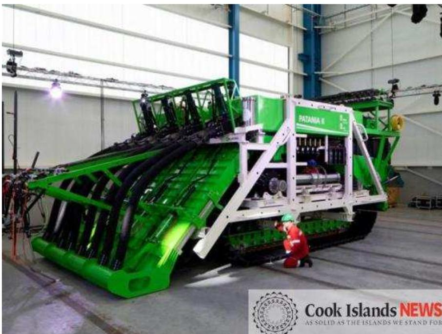
The Patania II, a scaled down prototype of a manganese nodule collector to be tested in 2019 in the Clarion Clipperton Zone.
